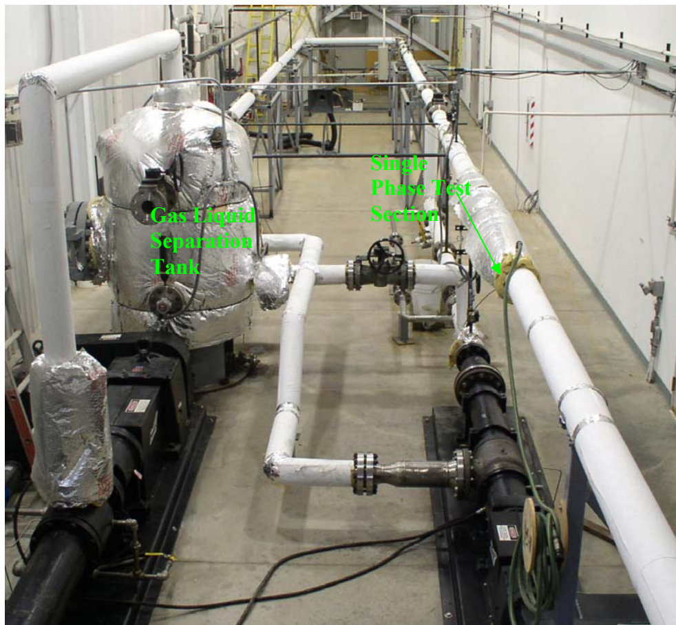
Figure 14. Hastelloy H 2 S flow loop.
